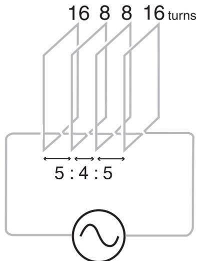
Fig. 1. Schema of coils of the facility for exposure to MFs. The actual facility had three sets of coils in X-, Y-, and Z-directions.
