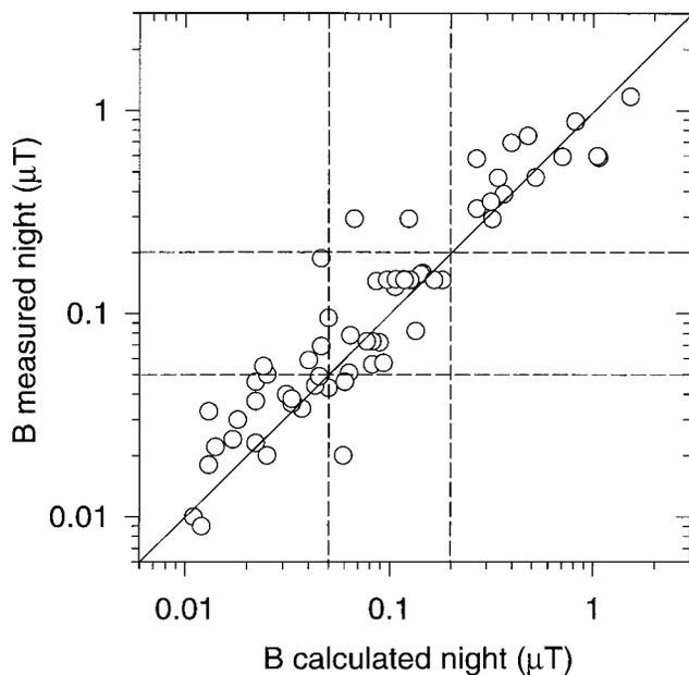
Fig. 5. Measured magnetic field (B) as a function of calculated magnetic field for night exposure only. For other details, see Figure 3.
