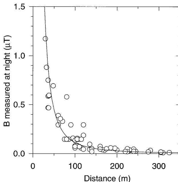
Fig. 2. Geometric means of individual magnetic fields (B) for the 65 children in the study, as a function from the distance to power line, for exposure at night only. No correction is made for differences in load on the power line. The solid line indicates the magnetic field calculated from the mean load during the measurements (night load, 354 A).
