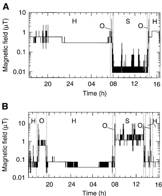
Fig. 1. Examples of magnetic field recordings with the Positron personal exposure instrument. In **A**, the child lived 60 m from the power line and attended a school about 300 m from the line. In **B**, the child lived 175 m from the power line and attended a school only 25 m from the line. H, at home; O, away from home; S, school.
