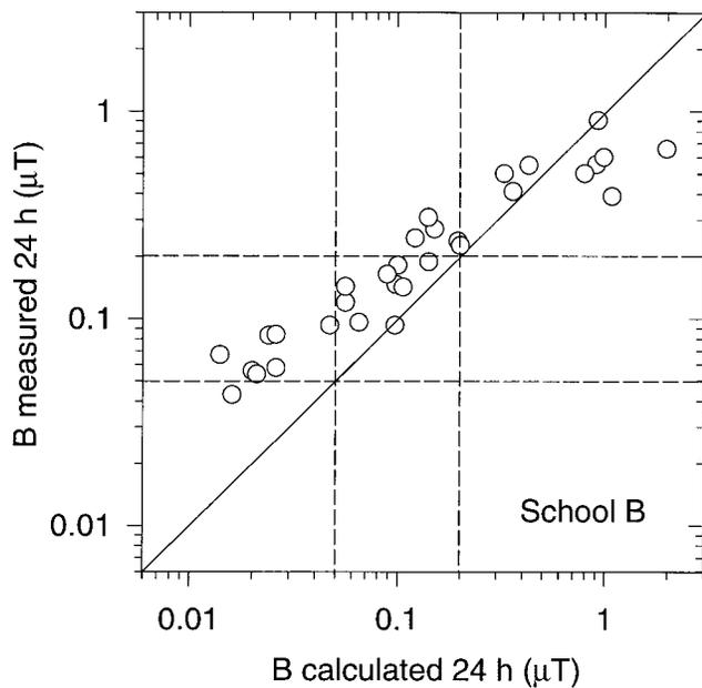
Fig. 4. Measured magnetic field (B) as a function of calculated magnetic field for 24 h exposure of 31 children attending a school located about 25 m from a power line. For other details, see Figure 3.
