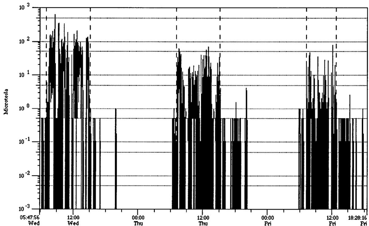
Fig. 2. Three days of measurement with a “high field” exposure meter (range, 1–7000 µT) same worker and measurement period as in Figure 1.
