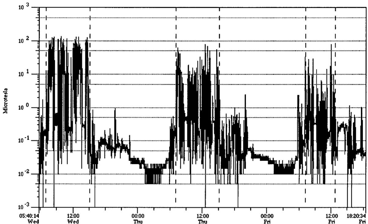
Fig. 1. Three days of measurement for a metal worker reporting: First day, 5 h of MMA welding; second day, 5 h of MIG/MAG welding; last day, 3 h of MIG/MAG welding. The vertical dashed lines indicate the beginning and finishing of work periods. The record comes from a "standard" exposure meter (0.01–70  $\mu\text{T}$  in three axis) and some overloading of the instrument is found in the first day of measurement.
